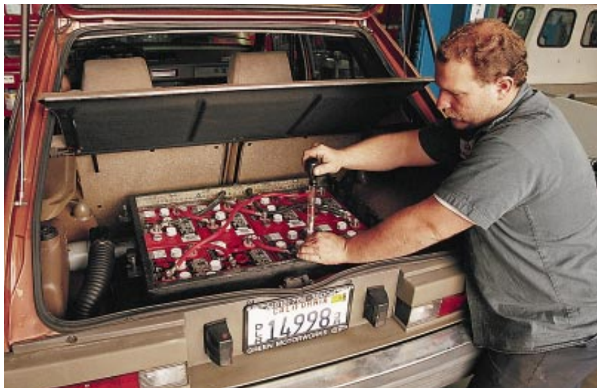
L.A. MECHANIC at Green Motorworks, a local manufacturer of electric vehicles, converts a gas-fueled car to battery power. Such initiatives are receiving strong support from California state agencies as a way to meet ambitious air-quality standards.
