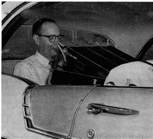
Fig. 1. Observer in rear seat of car can easily read meters of analyzers which are supported on the back of the front seat. Recorders may be installed in any convenient location.
