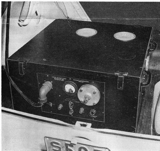
Fig. 3. Over-all view of the power pack as it is mounted in the trunk of the car. Carrying handles are provided for convenience. Cable at left feeds power to the analyzers.
